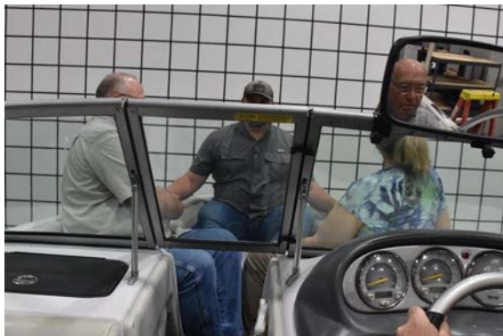
Visibility of 6' boat operator ( left ) vs 5'6" boat operator ( right ) from the driver's seat.
