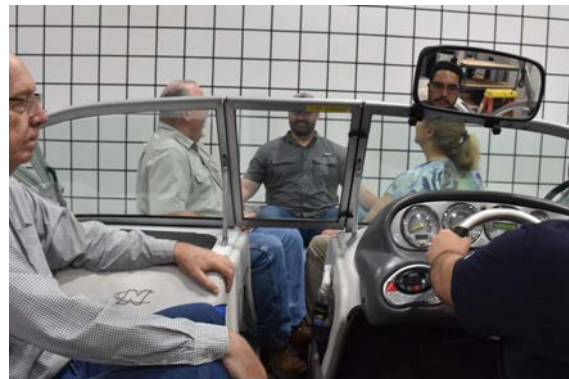
Visibility of 6' boat operator ( left ) vs 5'6" boat operator ( right ) from the driver's seat.
